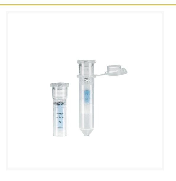
**Vivaspin centrifugal concentrators** offer the optimal solution for applications where protein solutions are concentrated or buffer solutions are exchanged. Through the membrane made of polyethersulfone (PES), their important macromolecules (e.g. proteins, DNA, antibodies, etc.) are retained, while unwanted by-products such as salts, solvents and small organic molecules pass through it. This ensures not only purification of the desired protein solution, but also its concentration.
