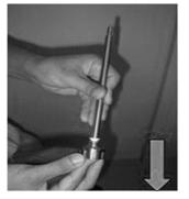
6. Remove the rotor from the stator by pulling in opposite directions
