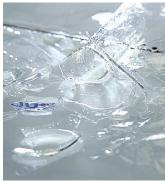
Volumetric flask without coating
