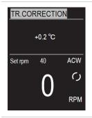
• TR.CORRECTION:Temperature sensing calibrator.(Range -10  $^{\circ}$ C -- +10  $^{\circ}$ C)
